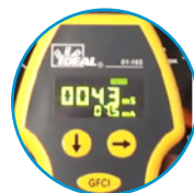
Trips GFCI at 6mA or 30mA
