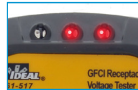
Red Lights Indicate Incorrect Wiring
