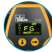
Detects and Displays false or "bootleg" ground
