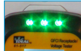
Green Lights Indicate Correct Wiring
